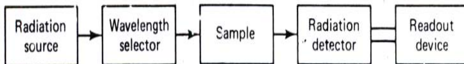
Figure 8.4: Basic components of a spectrometer
