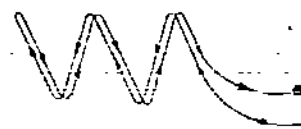
Fig. 2.4: Non-inductive winding. It is done for minimising the self inductance of the wire. The wire is doubled back on itself before being coiled up.
