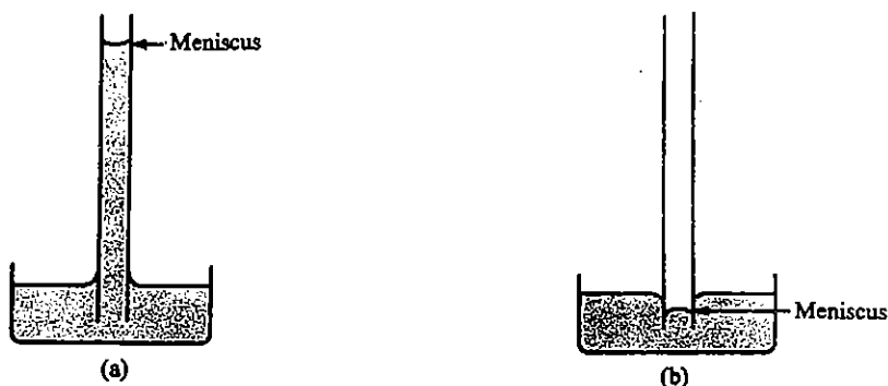
Fig. 4.3 (a) : A polar liquid such as water rises in a capillary tube—water has concave meniscus in a glass tube (b) : A metallic liquid such as mercury shows a depression of level—mercury has convex meniscus.
