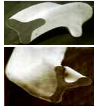
Cross-sectional views of nylon carpet fibers as seen with a scanning electron microscope (SEM)
